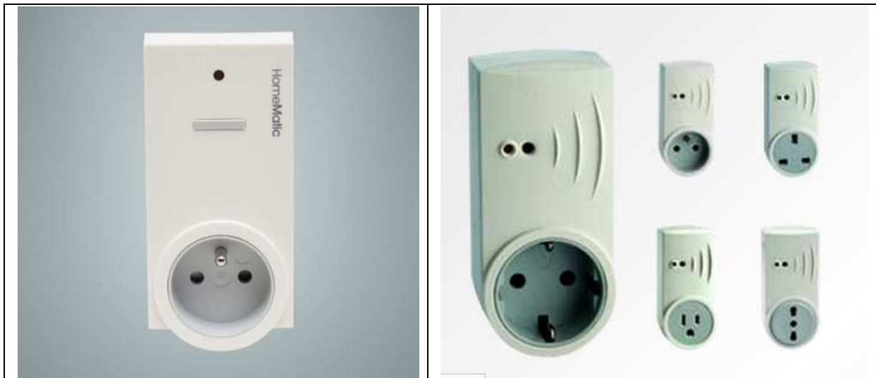
Figure 4: Left: Smart plug of type HomeMatic „Funk-Schaltaktor 1-fach mit Leistungsmessung, Zwischenstecker Typ E“ as used in Konstanz. Right: Smart plug of type 4-noks ZR-PLUG-XX-M, ZigBee electricity meter and remote control plugs as used in Caserta.
